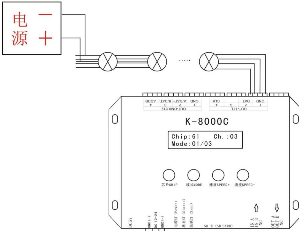
Single signal wiring diagram:
