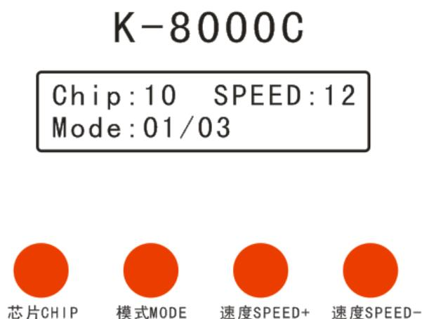
**Special Remarks:** Derived program after set one-key coding in the software, long press MODE for 5 seconds can write code to the lights directly, this function is very convenient and practical. Welcome to consult our engineer or salesman to learn the detailed operation method.
