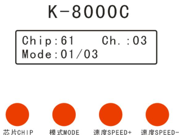
**NOTE:** 61 means UCS512A or B coding mode; 62 means WS2821 coding mode; 63 means SM DMX512AP; 64 means UCS512-C; Ch.: 03 means the coding channel is 3 channels
