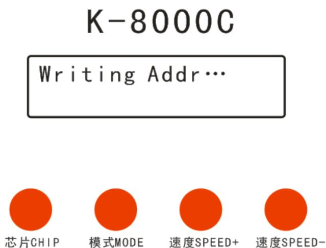
(3) After finished address code, press “CHIP” first and at the same time press “MODE” button, switch to playback mode, switch the chip to Chip: 10, this is the DMX512 standard agreement 250K playback mode. At this time, press MODE button and SPEED button can separately switch playback mode and adjust speed, as below:
